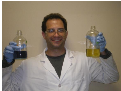
Blue Moly and Yellow Uranium rich eluates separated and recovered by Spiderweb column
